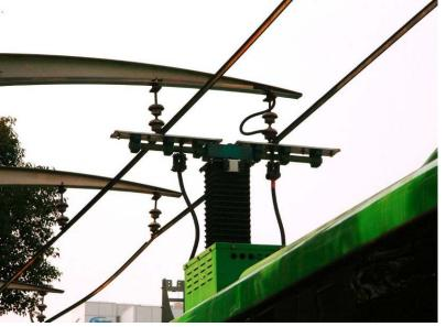
The bus uses ultra capacitor – charging faster than usual batteries.
