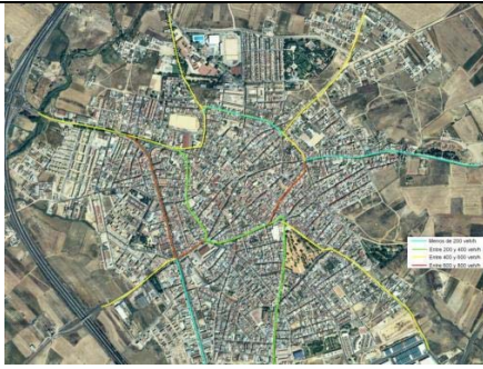
Traffic intensity in the primary road network in the town of Almonte
