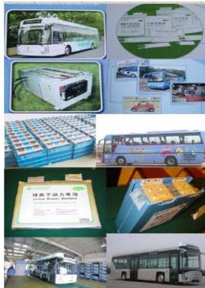
Figure III.7 LiMnO 2 Battery of MGL and the battery bus for Beijing Olympic Games.
